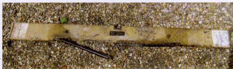
Right and above: A Berichtigungslatte with broken levelling bubble found recently on the cliffs near Essex Hill in Alderney
