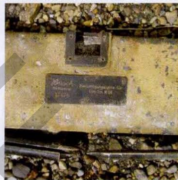
Right and above: A Berichtigungslatte with broken levelling bubble found recently on the cliffs near Essex Hill in Alderney
